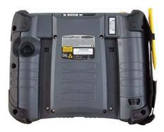
much as four working days under depending upon operating conditions. That's pretty phenomenal. To remove or replace it, you turn a spring-loaded thumbwheel until the battery pack is released. With this kind of battery life, take a spare with you and you never have to worry about finding an outlet.
