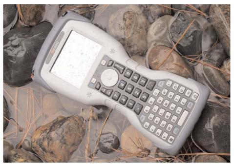
the familiar functionality of a standard keyboard. Keys are color-coordinated by function, and there is a large and correctly placed 9-way directional button that can be used instead of, or in conjunction with, the touch screen. ALT, 2nd, CTRL, and Shift are implemented as "sticky keys," providing access to additional functions. All keys provide tactile feedback and the keyboard bezel is removable for cleaning without affecting the seal.
