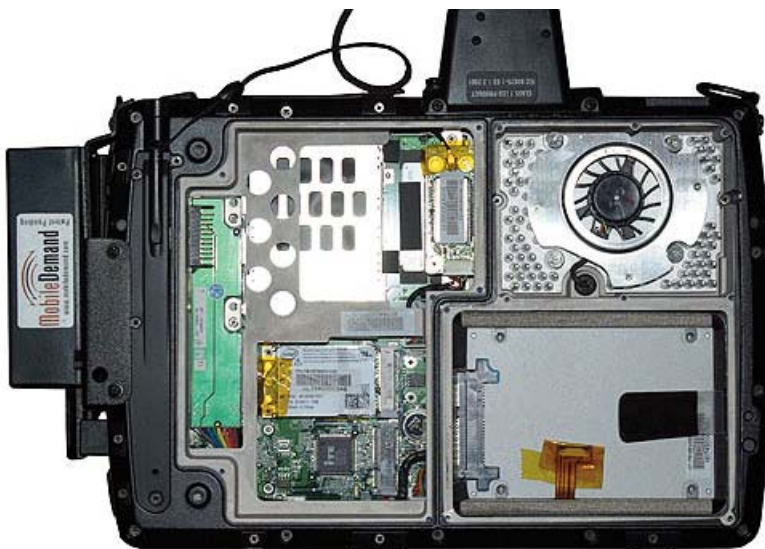
Backside with protective covers removed: solid structural design
